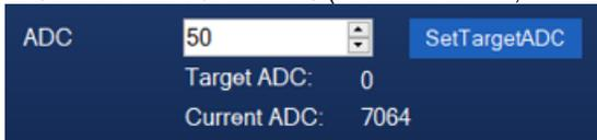
Type the target ADC value in the number box and click "SetTargetADC" button to set TargetADC value of device. The device would automatically modify the voltage to maintain CurrentADC to match TargetADC.
