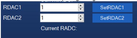
Set RDAC1 and RDAC2 value in number box and click "SetRDAC1" and "SetRDAC2" buttons to set the RDAC value. RDACx works as the gain of Feedback control. The bigger the value of RDAC, the attenuation range of VOA would be larger. RDAC1 and RDAC2 can be set a value between 1 and 1023.
